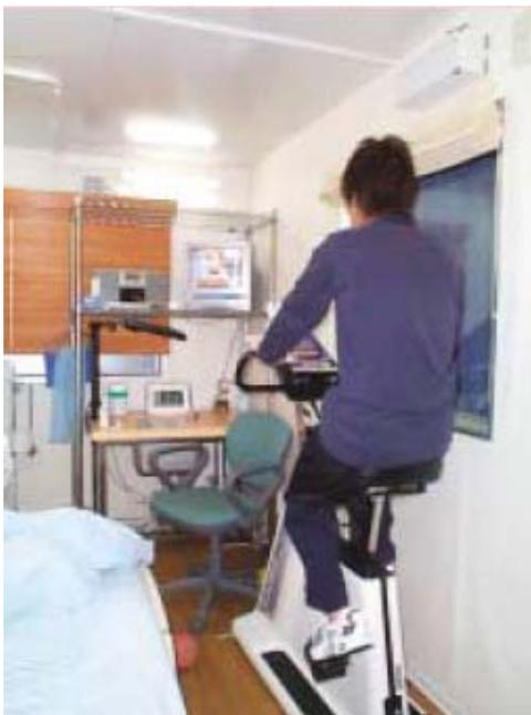
Now, these problems have been sorted out by the introduction of human calorimeter, as its measurement error can be kept within  $\pm 1\%$  (quite lower than that of earlier methods) for long hours, even for several days, by checking it with regular alcohol combustion test. Furthermore, it is also possible to estimate the expended energy sources (e.g. carbohydrate, lipid, protein).
